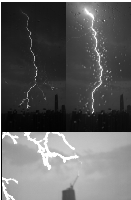
Figure 1. High-speed camera records of a downward negative flash struck a structure about 90 m high. Fig. 1a and 1b are captured at a sampling rate of 7,000 fps
