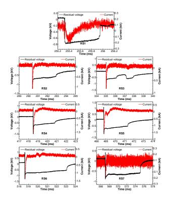
Fig.2 Waveforms of residual voltage and current through the SPD and corresponding to the first seven return strokes.
