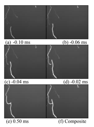
Fig.1 High-speed images of F1111 captured by the high-speed camera with a sampling of 50,000fps. Fig. 1f is the composite image of 75 images before the return stroke and the image 0.5 ms after the return stroke.
