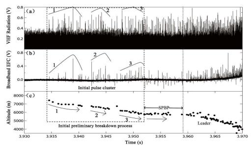
**Fig. 1** The initial preliminary breakdown process of negative CG flash 201503: (a) VHF radiation (relative value), (b) broadband electric field change (relative value), and (c) mapping altitude of the radiation sources.
