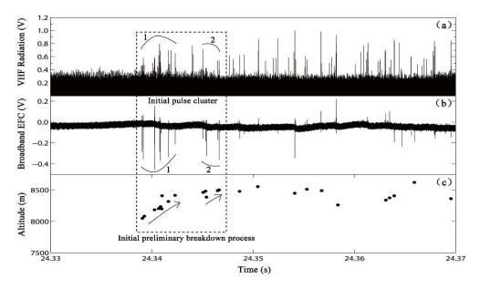
**Fig. 6** Negative CG flash 201124: (a) VHF radiation (relative value), (b) broadband electric field change (relative value), and (c) mapping altitude of the radiation sources.
