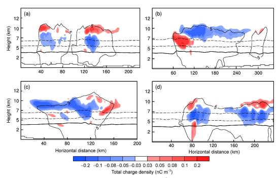
**Fig. 2** Vertical cross-sections of total charge density (nC m<sup>-3</sup>; shaded). The horizontal lines represent the isotherm lines of 20, 10 (dashed line), and  $0^{\circ}$ C (solid line). The solid line labeled "5" represents the contour line of 5 dBZ.
