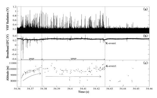
**Fig. 4** The preliminary breakdown process of the second category of IC flashes, showing the synchronized charge for the radiation sources in flash 210954 (54.36–54.46 s): (a) the VHF radiation (relative value), (b) the broadband electric field change (relative value), and (c) the altitude.
