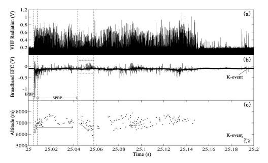
**Fig. 3** The preliminary breakdown process of the first category of IC flashes, showing the synchronized charge for the radiation sources in flash 205725 (25.00–25.20 s): (a) the VHF radiation (relative value); (b) the broadband electric field change (relative value); and (c) the altitude.
