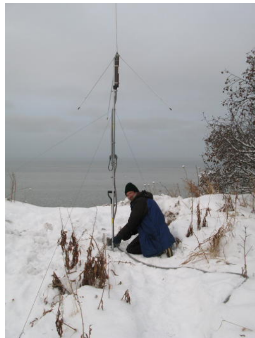
Setting up portable mapping stations on Kenai Peninsula coast overlooking Cook Inlet, used to study Redoubt Volcano eruptions. Above: Paul Krehbiel working on station electronics. Right: Ron Thomas setting up VHF receiving antenna. Redoubt is in background obscured by ever-present clouds.
