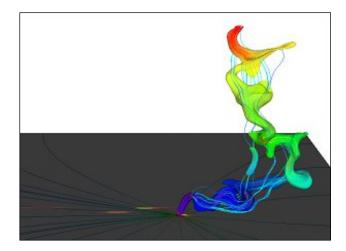
Computation of a 6000K iso surface of a 50cm arc attached on a metallic plate. The electrical potential of the arc is color coded from 0 to  $\sim$  400V.
