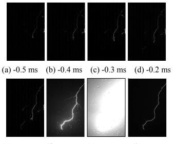
(e) -0.1 ms (f) 0.0 ms (g) 0.1 ms (h) 0.5 ms Fig. 1 High-speed camera records of L01. In frame a-e, luminosities are enhanced for a better view.
