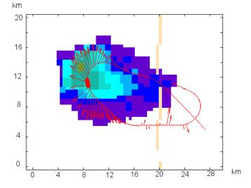
The red arrow indicates the direction and magnitude of the horizontal field (maximum value  $\sim 12kV/m$ ) at 6250m AMSL superimposed on the trajectory of the aircraft and the precipitation radar echo at about 2500m AMSL.
