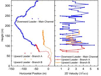
Fig.2 The 2D spatial positions (Left) and propagation velocities (Right) of the main channel
