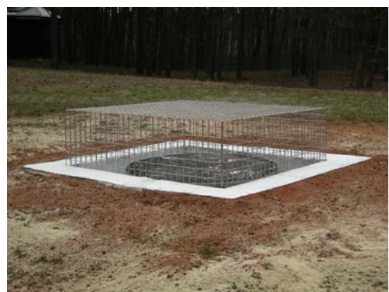
Figure. 1. Screened Wilson antenna prepared for the purpose of convection current density measurements at Swider station.
