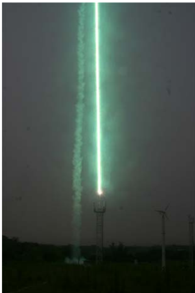
Fig.1 Lightning flash triggered at 180026 on 30 July 2011. This lightning directly stroke the iron tower mounted with wire communication transmitting equipment. The wind generator is shown in the right of this photograph.
