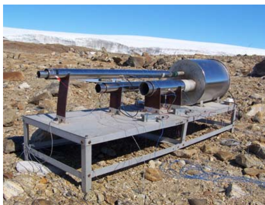
Figure: 1. Gerdian Ion Counter Battery installed at the Indian Antarctic station Maitri designed and fabricated by IITM Workshop.
