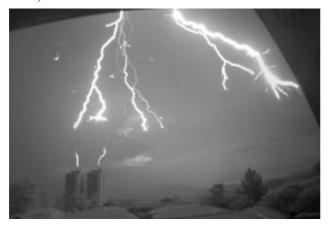
Figure 2 – Frame from high-speed video showing the upward connecting leaders from buildings in response to a negative CG flash (9 February 2014).
