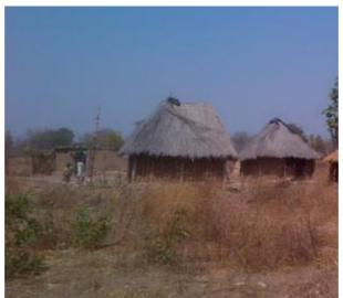
Fig 1 – Typical housing and work structures in developing countries involve mudbrick walls with a combination of flammable thatch and ungrounded metal roofs, often held down by stones. (courtesy Mary Ann Cooper)
