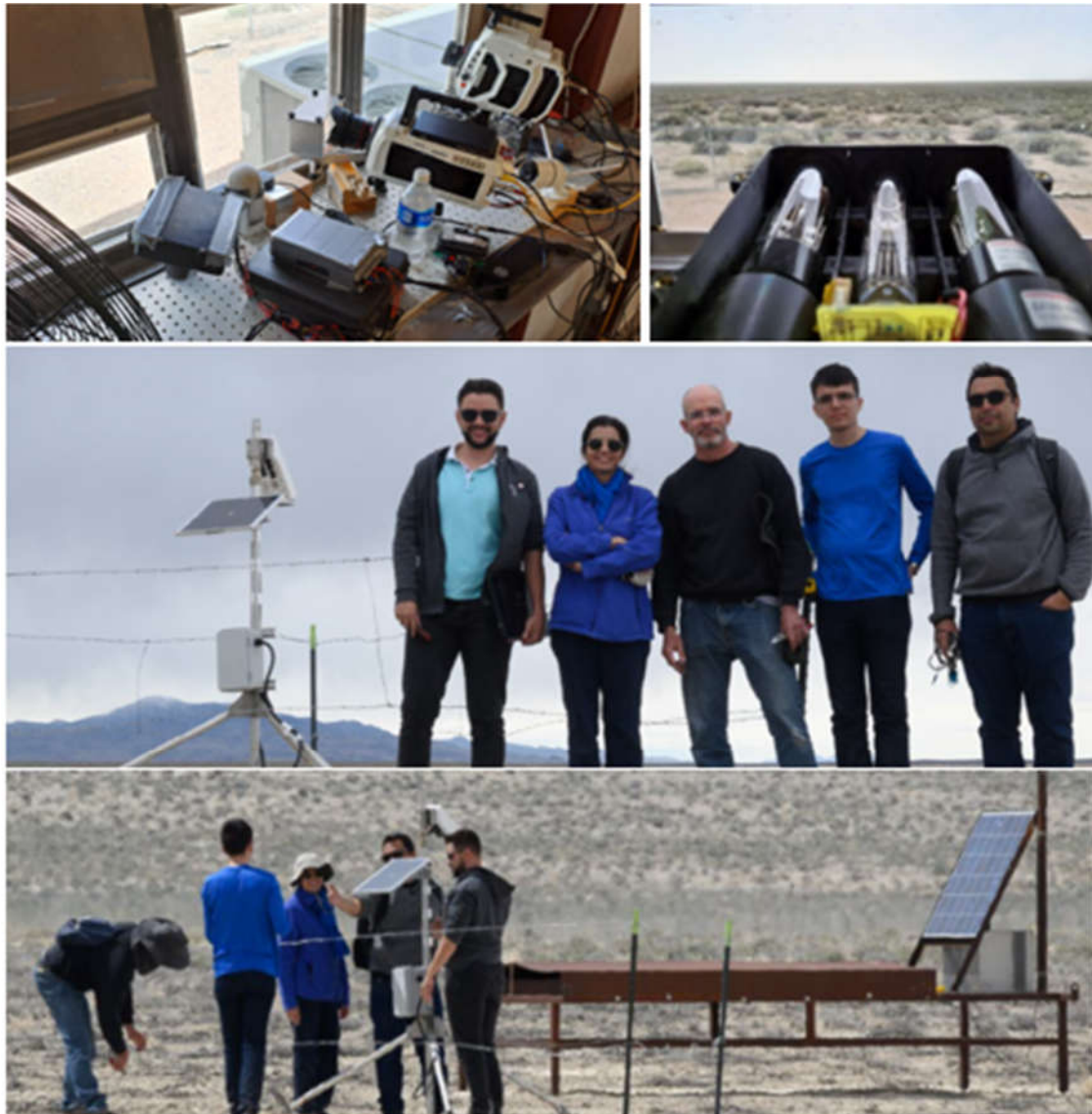
Figure 1. High-speed cameras, photometers, electric-field mill, and the gamma ray detector in Utah.
