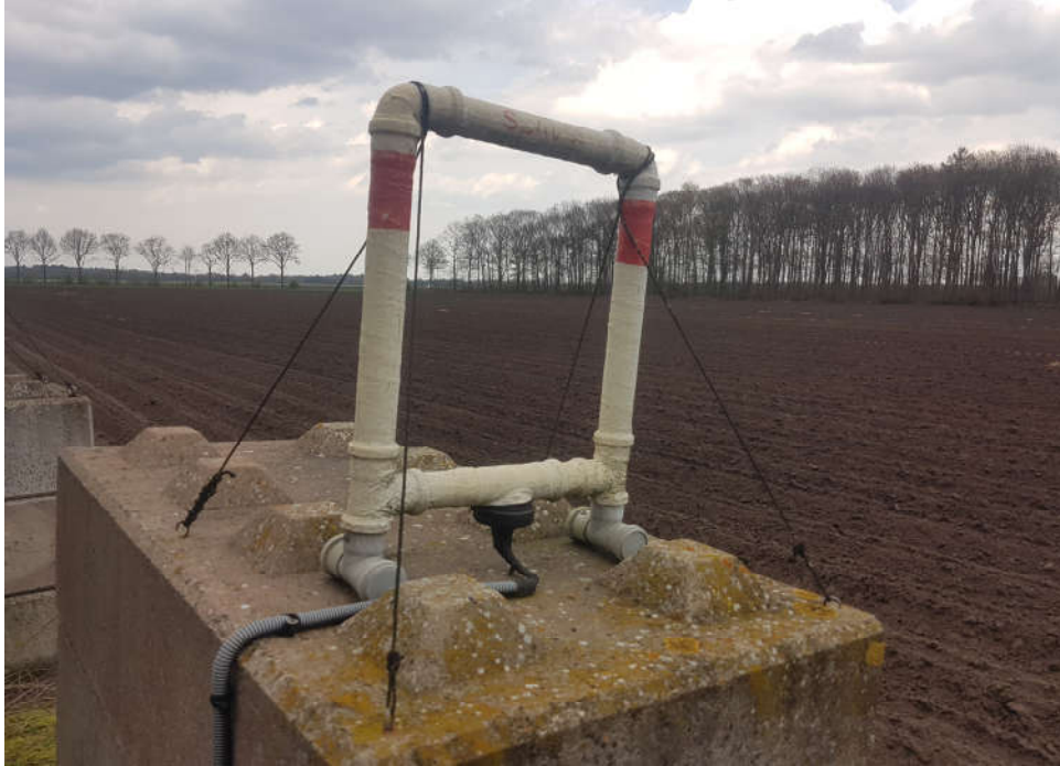
Figure 1. Broadband shielded magnetic loop with an integrated preamplifier installed close to Ter Wisch, Netherlands.
