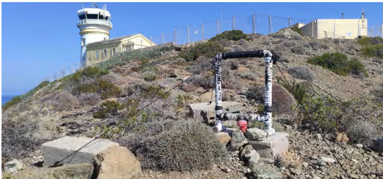
Figure 1. Broadband shielded magnetic loop with an integrated preamplifier installed at Cap Corse, Corsica, France.
