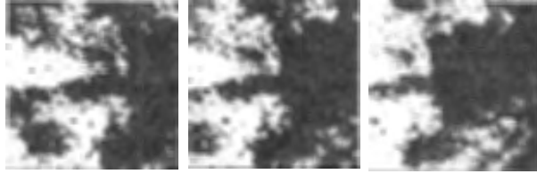
Fig. 1 First, third and the fifth images from set of ten modeled images with 256 \times 256 pixels and \Delta x = \Delta y = 1m , \Delta t = 1s , simulating non-uniform linear motion from right to left with mean DV V_{mod} = -25.22 m/s .
