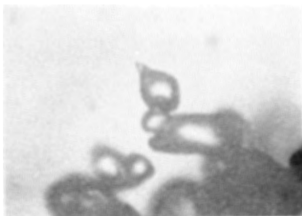
C. A droplet of about 25\mu\text{m} diameter showing a protuberance collected at a speed of 1.75\text{m s}^{-1} and temperature -7\frac{1}{2}^{\circ}\text{C}
