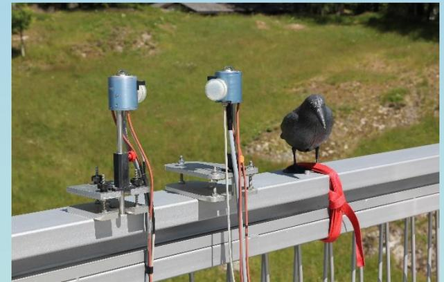
Input Optics of the two reference spectroradiometers QASUME and QASUMII
