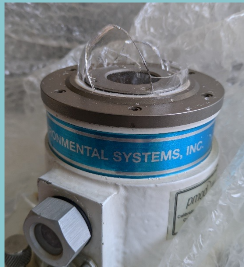
Input Optics of the two reference spectroradiometers QASUME and QASUMEL
